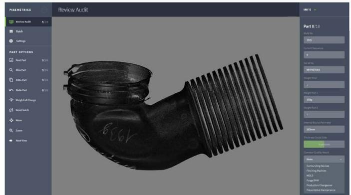
Figure shows Relimetrics user interface analyzing dimensions and surface defects of a blow molded plastic part.
